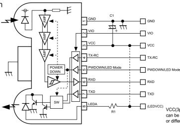
VCC(3pin),VIO(2pin) and LEDVCC(8pin) can be used on either common power source or different one
