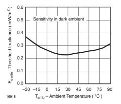
Figure 10. Sensitivity vs. Ambient Temperature
