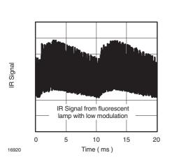
Figure 14. IR Signal from Fluorescent Lamp with low Modulation
