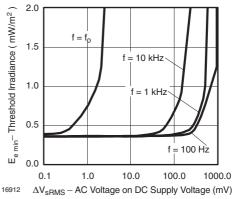
Figure 7. Sensitivity vs. Supply Voltage Disturbances
