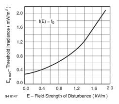
Figure 8. Sensitivity vs. Electric Field Disturbances
