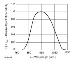
Figure 11. Relative Spectral Sensitivity vs. Wavelength
