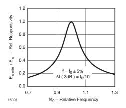
Figure 5. Frequency Dependence of Responsivity
