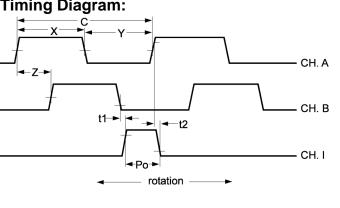
CPR (N): The number of Cycles Per Revolution. One Shaft Rotation: 360 mechanical degrees, N cycles.
