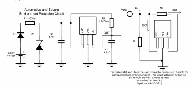
If reverse supply protection is desired, use a resistor in series with the  $V_{DD}$  pin. The resistor will limit the supply current (Fault),  $I_{DD}$ , to 50 mA. For severe EMC conditions, use the application circuit on this page.
