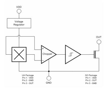
**Note**: This is a static-sensitive device. Please observe ESD precautions. Reverse VDD protection is not included. For reverse voltage protection a 100Ohms resistor in series with VDD is recommended.
