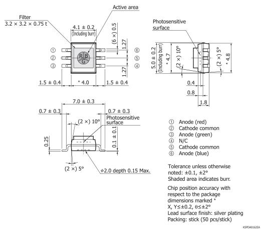
Note: If excessive vibration is continuously applied to the glass filter, there is a risk that the filter may come off, so secure the glass filter with a holder.
