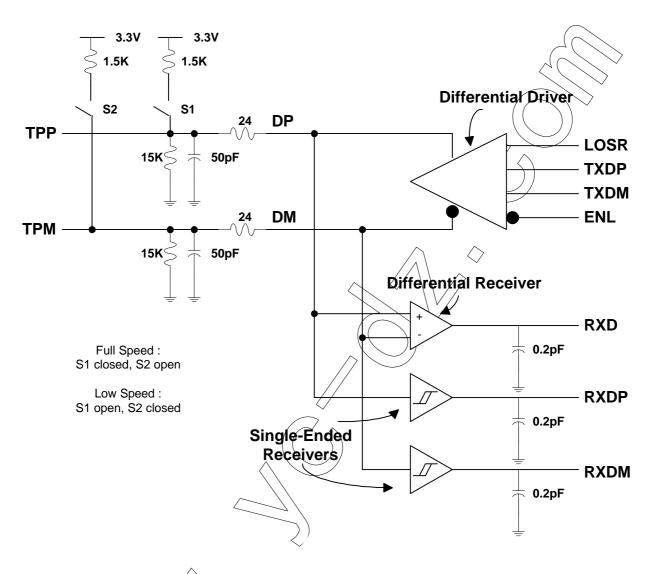
The following figure describes the key parameters of the differential driver – values for these parameters for high and low speed operation are listed in the tables overleaf. The abovefigure includes details of the loading for this testing.
