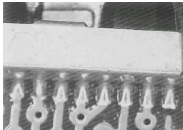
Photo 4.0. Unit self-aligns after reflow.
