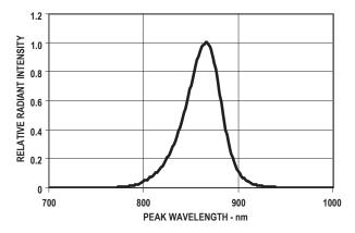
Figure 1. Peak Wavelength Vs Relative Radiant Intensity
