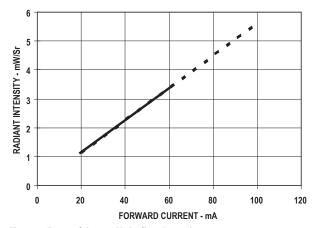
Figure 3. Forward Current Vs Radiant Intensity
