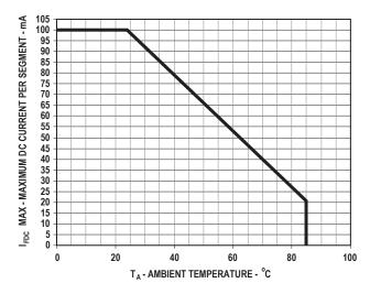
Figure 5. Forward Current versus Ambient Temperature derated based on Tj - 110  $^{\circ}$ C and thermal resistance at 380  $^{\circ}$ C/W
