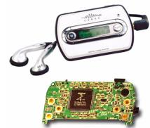
\* 2xAA, 2xAAA and Li-lon configurations require 144-pin package. Li-lon is supported with 100-pin package but several external components are required. MPEG Layer 3 audio coding technology licensed from Fraunhofer IIS and THOMSON multimedia.
