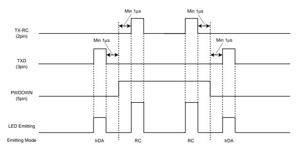
\*If TX-RC or TXD input pulse width is wider than 48µs, output LED emitting pulse will be turn off approximately 48µs.
