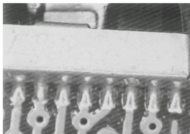
Photo 4.0. Unit self-aligns after reflow.
