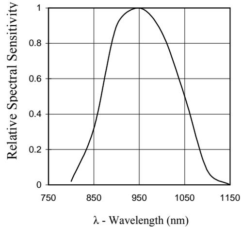
RELATIVE SPECTRAL SENSITIVITY vs. WAVELENGTH
