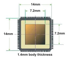
The form factor of the EntréPad AES3500 is 100-pin JEDEC-standard Low-profile Quad Flat Package (LQFP)
