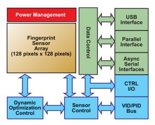
The EntréPad AES3500 sensor incorporates flexible Select-a-Bus™ architecture. This feature allows the developer to deploy designs that use not only the popular Universal Serial Bus, but also asynchronous serial interfaces and an 8 bit parallel interface implementation.
