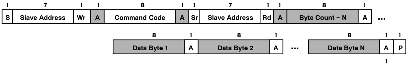
Figure 15. SMBus Block Read or I 2 C Read (Combined Format) Protocols
