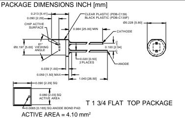
**DESCRIPTION:** The **PDB-C139** detector is a 4.10 mm<sup>2</sup> planar pin photodiode packaged in a T 1 3/4,flat top, water clear plastic housing. Designed for high speed, low capacitance, photoconductive applications. The **PDB-C139F** includes a daylight filter.
