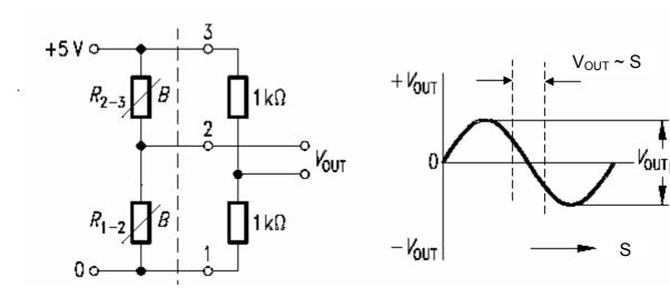
To convert small distance into a proportional electric signal, one can use a small soft iron part with definite width (e.g. b=1.8mm) to move over the face of the sensor. A linear signal up to 1.5mm can be obtained in this way. The sinusoidal signal gives a voltage output proportional to the distance in the zero crossover region.
