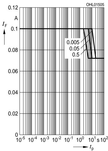
**Zulässige Impulsbelastbarkeit  $I_F = f(t_p)$** **Permissible Pulse Handling Capability**Duty cycle  $D$  = parameter,  $T_A = 85^{\circ}\text{C}$
