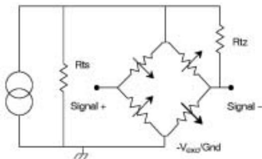
Figure 9. Simplified Compensation Circuit for TCZ and TCS Correction
