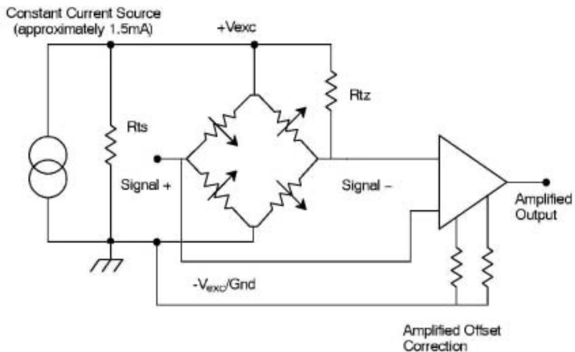
Figure 8A. Offset Correction Approach for SM5310, SM5415, and SM5455
