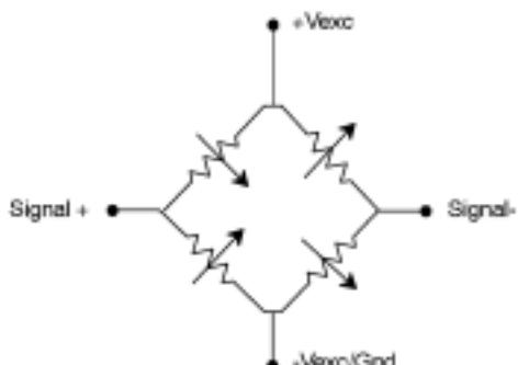
Figure 1 - 5310, 5415, and 5455 Equivalent Circuit
