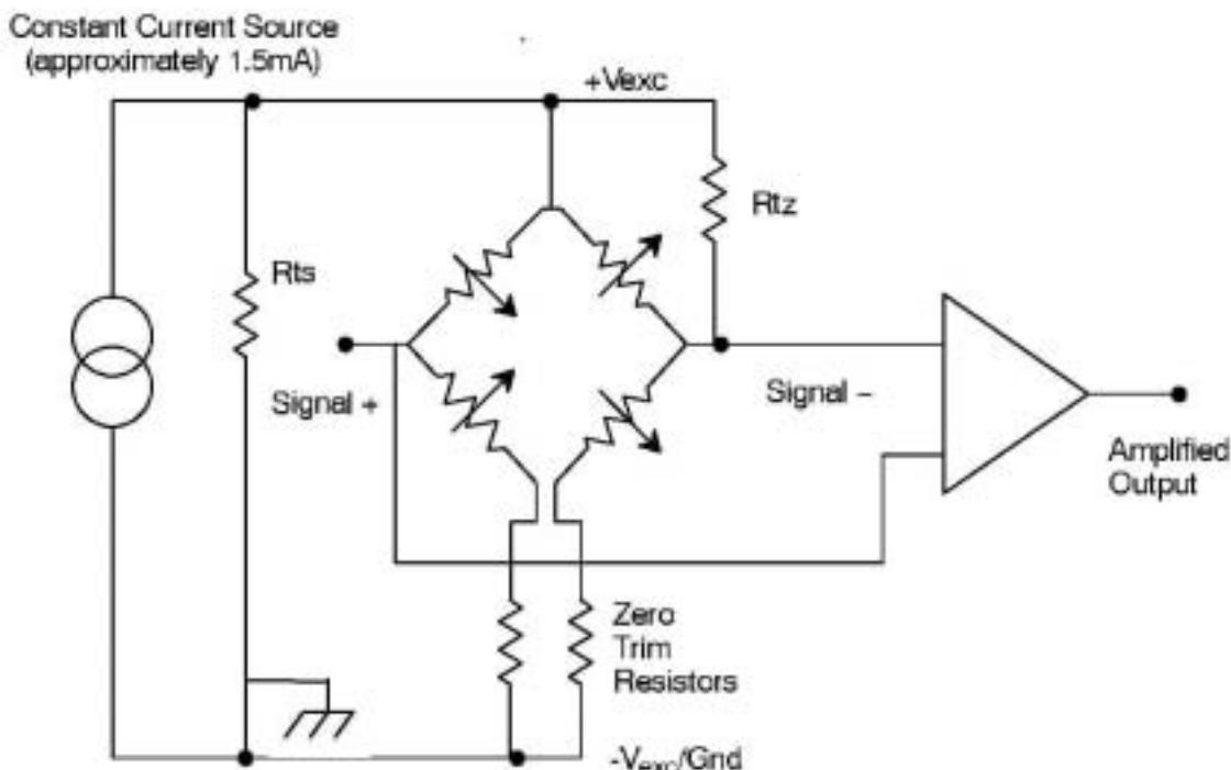
Figure 8B. Offset Correction approach for SM5410, SM5350, and SM5450
