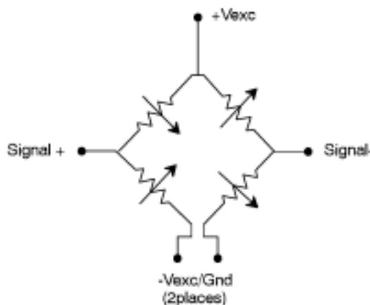
Figure 2 - 5350, 5410, 5450 Equivalent Circuit
