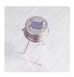
The DigiPyro® PYD 1978, with its 3 x 4 mm<sup>2</sup> window size, provides you with a low-cost digital solution to motion detection.
