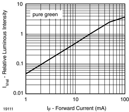
Figure 5. Relative Luminous Intensity vs. Forward Current
