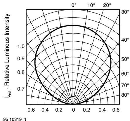
Figure 2. Rel. Luminous Intensity vs. Angular Displacement
