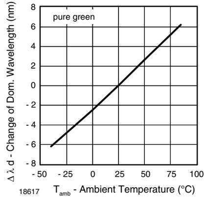
Figure 7. Change of Dominant Wavelength vs. Ambient Temperature
