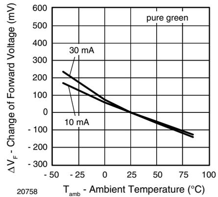
Figure 8. Change of Forward Voltage vs. Ambient Temperature
