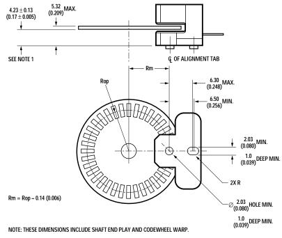
ALL DIMENSIONS FOR MOUNTING THE MODULE/CODESTRIP SHOULD BE MEASURED WITH RESPECT TO THE TWO MOUNTING POSTS, SHOWN ABOVE.
