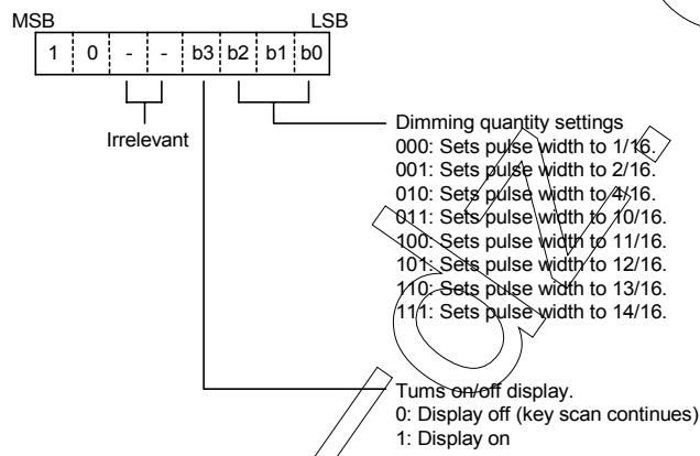
On power application, the 1/16-pulse width is set, the display is turned off and key scanning is stopped.
