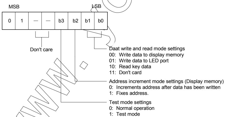
Note: For power application, the normal operation and address increment modes are set.
