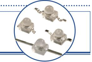
The OP270 series are GaAlAs infrared LEDs mounted in a clear plastic SMT packages. The devices incorporate an integral molded lens which enables a narrow beam angle and provides an even emission pattern. This series is available with four lead configurations and is compatible with most automated mounting equipment. The OP270 Series LEDs are mechanically and spectrally matched to the OP570 series phototransistors.
